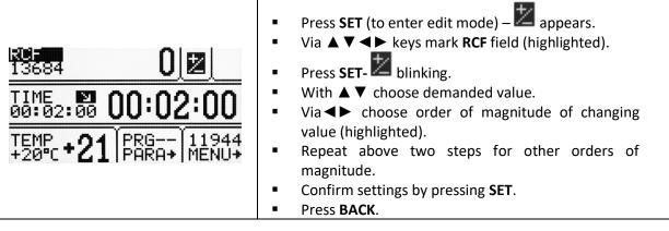
When RCF is changed, RPM is automatically corrected.
