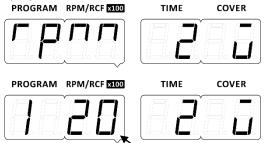
The **RPM** value is displayed without a dot (picture above), while the **RCF** value is shown with a dot as in the image below.
