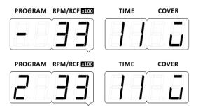
The program is edited with the direction keys 💽 🔽 under the appropriate set field - (RPM / RCF)
