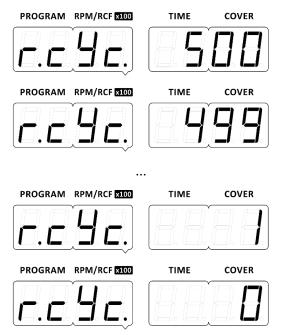
After exceeding 70000 rotor operation cycles (the value of 0 in "**r.cYc.**" will appear) or **10 years** after the purchase of the device or the rotor with accessories, **it is absolutely necessary to replace the rotor and its accessories due to wear**.
