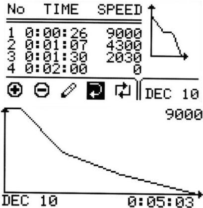
After programming the time value, you can graphically display the **TIME + SPEED** segment of the user's braking characteristic. The set section of the characteristic curve is illustrated on the graph, which can be displayed by selecting
