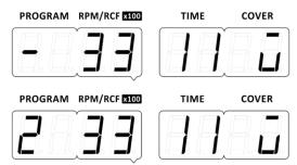
The program is edited with the direction keys ▲ and ▼ under the appropriate set field - (RPM / RCF)
