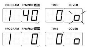
The stop of the rotor from the program is signaled by the simultaneous flashing of the **RPM / RCF** and **TIME** values. Flashing in the picture is marked by dashes deviating from the appropriate parameter. When the speed reaches zero, the lid is automatically opened (if so, set in the advanced
