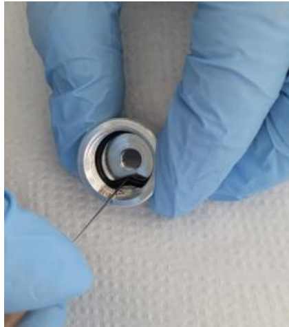
Fig. 25. Removal cap gasket by needle.
