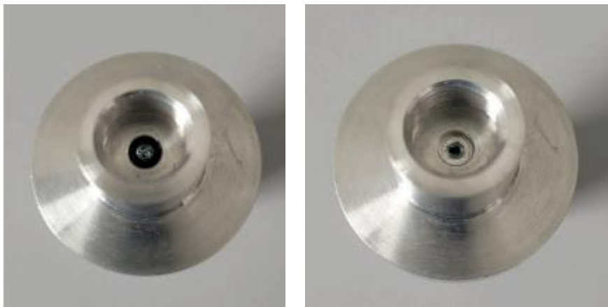
Fig. 26. Before and after removal of thread of the nozzle gasket.
