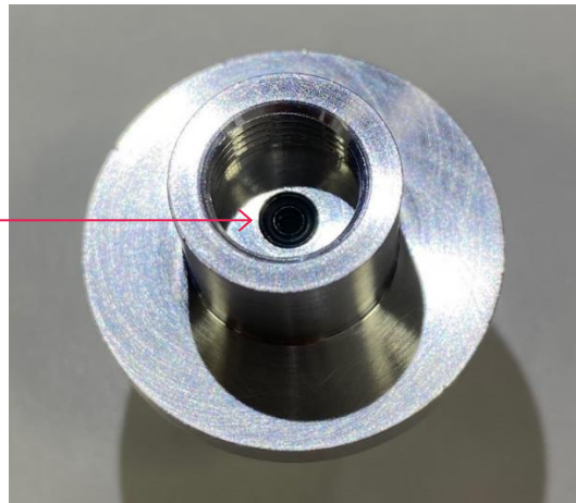
Fig. 2. Correctly installed nozzle seat gasket
