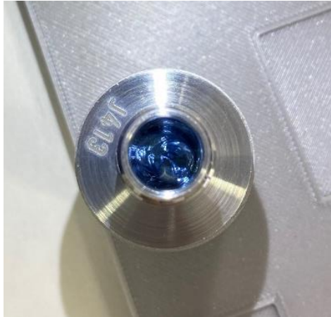
Fig. 6. Cartridge filled with paste prior to centrifuging, with clean cylinder walls.
