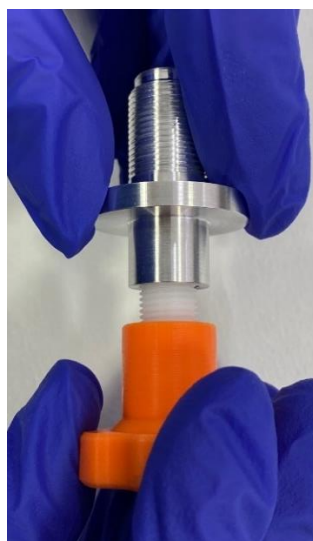
Fig. 3. Nozzle seat assembly with the help of the wrench.
