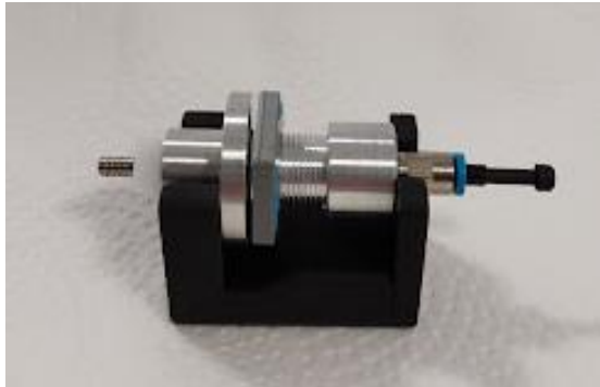
Fig. 19. Correctly tightened cartridge
