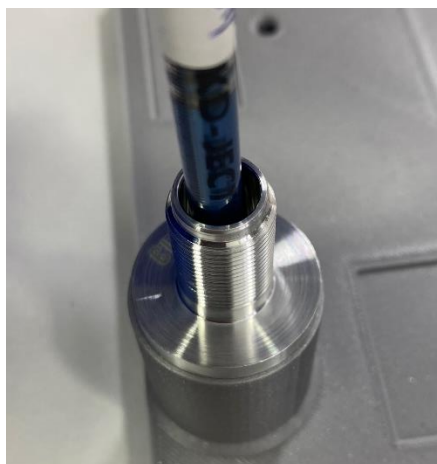
Fig. 5. Filling of the cartridge from the syringe
