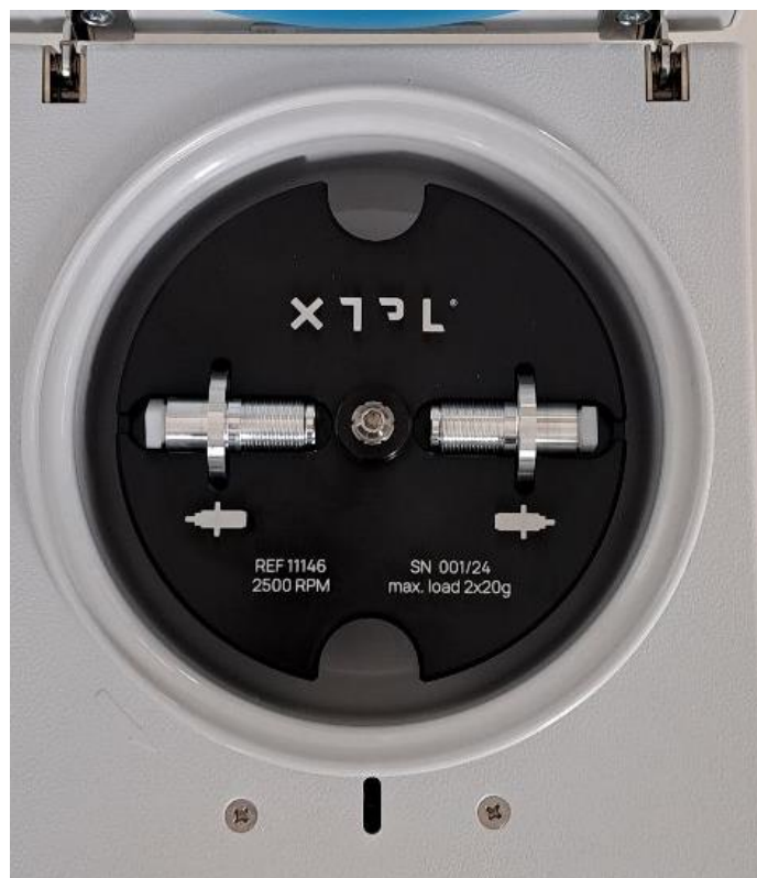
Fig. 21. Cartridge and counterweight (or second cartridge) correctly placed.
