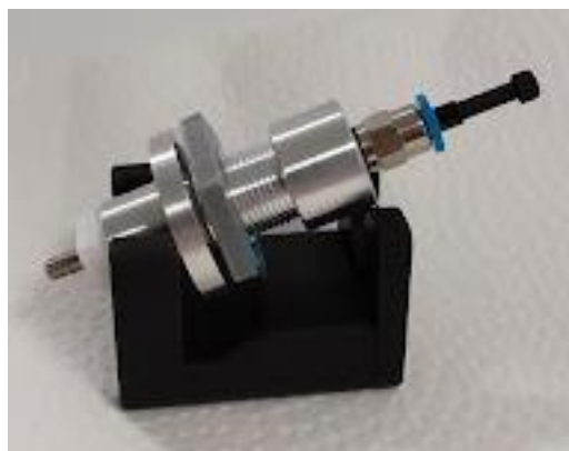
Fig. 20. Incorrectly tightened cartridge will not fit into the gauge.
