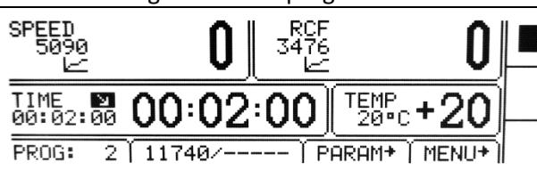
Icon signals that program with user acceleration/deceleration characteristics are loaded.
