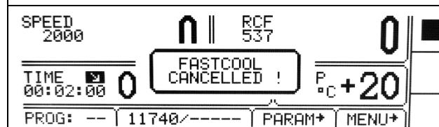
It is possible to exit **FAST COOL** mode at any time by pressing **STOP** key.
