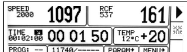
**FAST COOL** mode is marked by symbol XX XX blinking in the right upper side of display.
