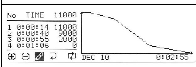
After programming the time and / or speed values, the segment (all segments) is graphically displayed on the graph on the right side of the screen. The time value is on the horizontal axis of the user's braking characteristic, while the speed is on the vertical axis.
