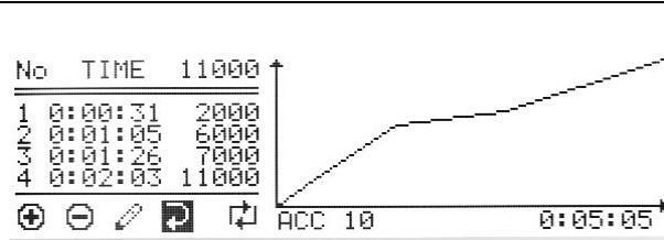
After programming the time and / or speed values, the segment (all segments) is graphically displayed on the graph on the right side of the screen. The time value is on the horizontal axis of the user's starting characteristic, while the speed is on the vertical axis.
